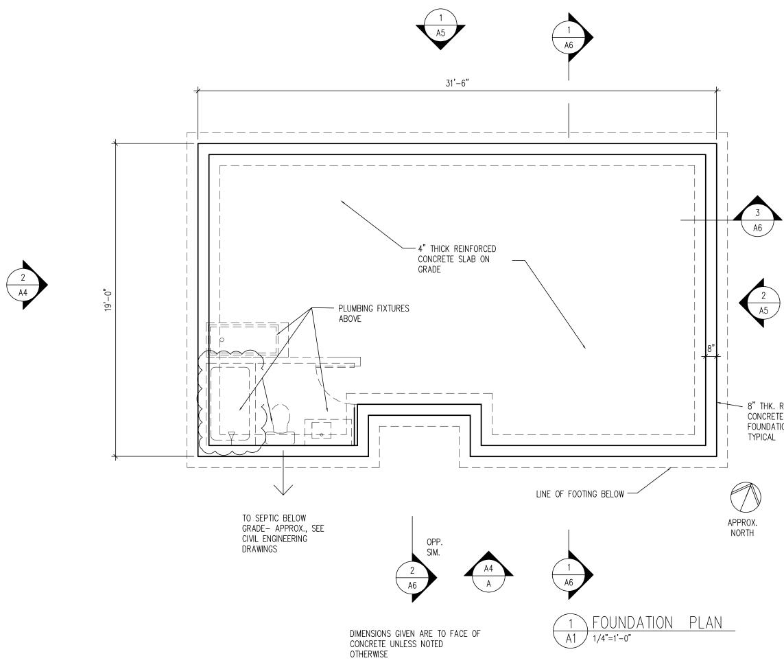
8" THK. REINF. CONCRETE FOUNDATION WALL
