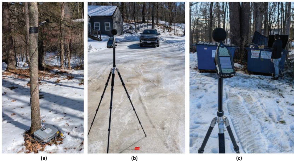
Figure A-1. Installed 7-day sound monitor (a), sound measurement of car door slam, horn, and engine start (b), dumpster lid slam impact sound measurement (c) Wake Robin Inn, Salisbury, CT
