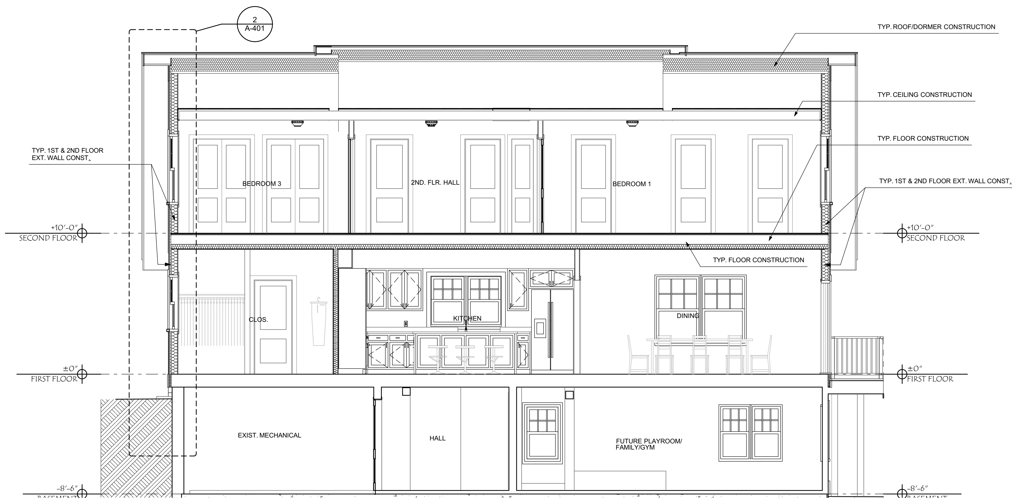
3 A-301 N-S BUILDING SECTION SCALE: 1/4" = 1'-0"
